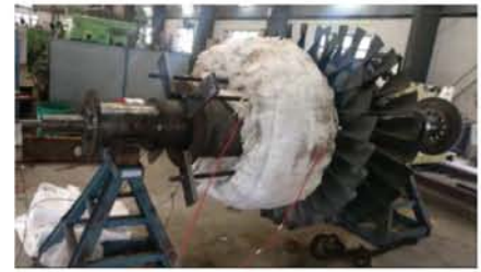
Blades removal by drilling Front drum removal by Induction heating
