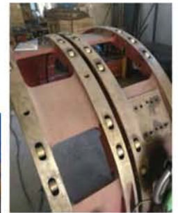
Regulating ring with Rollers & pins assembled
