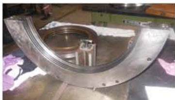
Carbon glands inspection
