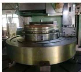
New sealing sleeve machining
