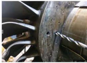
Blades removal by drilling Front drum removal by Induction heating
