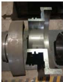
Sealing sleeve casting
