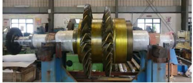
Rotor after repair with new blades in assembled
