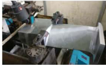
Blade root wire cutting
